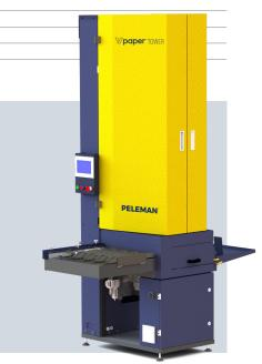
The V-Twister has been designed to turn your double-sided printed or printable paper into lay-flat pages, one by one. Through a single-step process, our innovative technology forms the paper fibres for each sheet, creating a supple hinge at the spine of the book. This makes your publication lay open effortlessly.
